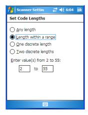
Choosing *One discrete length* allows you to decode only those codes containing a selected length. Choosing *Two discrete lengths* allows you to decode only those codes containing two selected lengths. *Length within a range* allows you to decode a code type within a specified range from 1 to 55.
